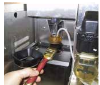
Clean the piston filter with the brush, and a wet cloth.
