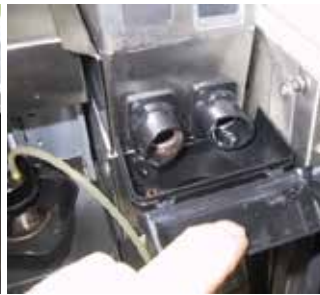
Flip open mixer lids and clean with the small brush
