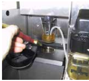
Clean the area behind and in front of the brewing chamber with the brush
