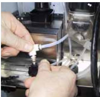
Pull the clip to release the steam nozzle
