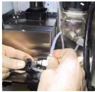
Lift up steam nozzle, and clean nozzle hole with the clip.
