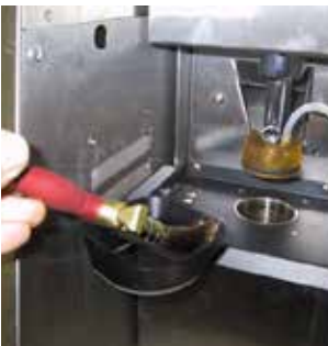
Clean the scraper with the brush
